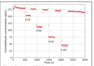
Fig. 1. Evolution of  $CH_2O$  concentration while varying the voltage applied to the  $\mu DBD$ , for 2, 3, 4, and 5 kV.
